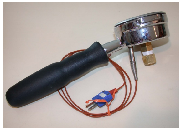
Figure 2. Portafilter thermometer side view showing the thermocouple probe's exit through the bottom of the portafilter, and the brew water metering orifice.
